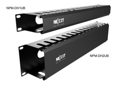
Nexxt Solutions horizontal Duct cable management is designed to be mounted onto any standard 19-inch EIA rack or cabinet. Fingers have smooth edges and are widely spaced to give additional cable support, also allowing terminated wires to be installed, removed or rerouted easily. Its innovative cover provides full access to cables, while improving the appearance of panels by keeping small and large bundles of cords neatly organized.
