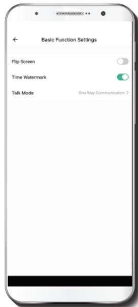
**Flip screen:** flips the image 180 degrees, if the camera is mounted upside down.
